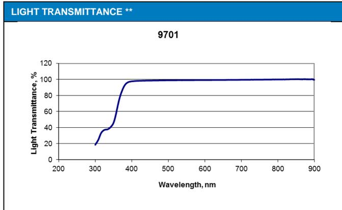
\*\* Measured at 0.03 mm [0.001in] per DSTM-501‡
